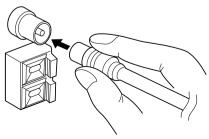
If reception is poor, connect the outdoor antenna.
